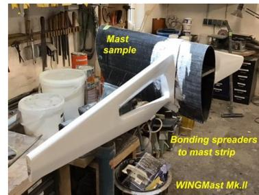
The Mk.II also shows a streamlined spreader design for less air drag.
